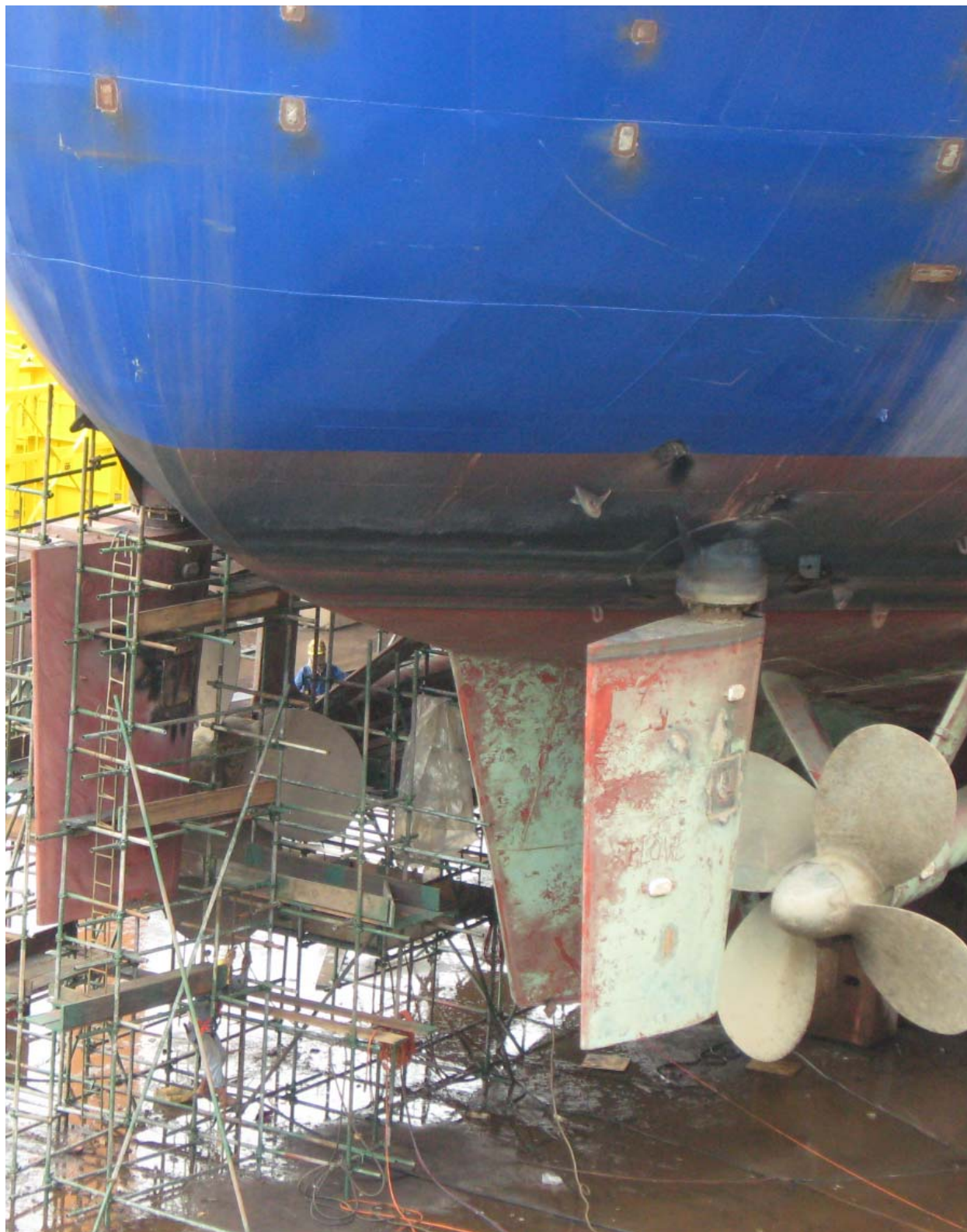
Removing ship propellers in dry dock.
