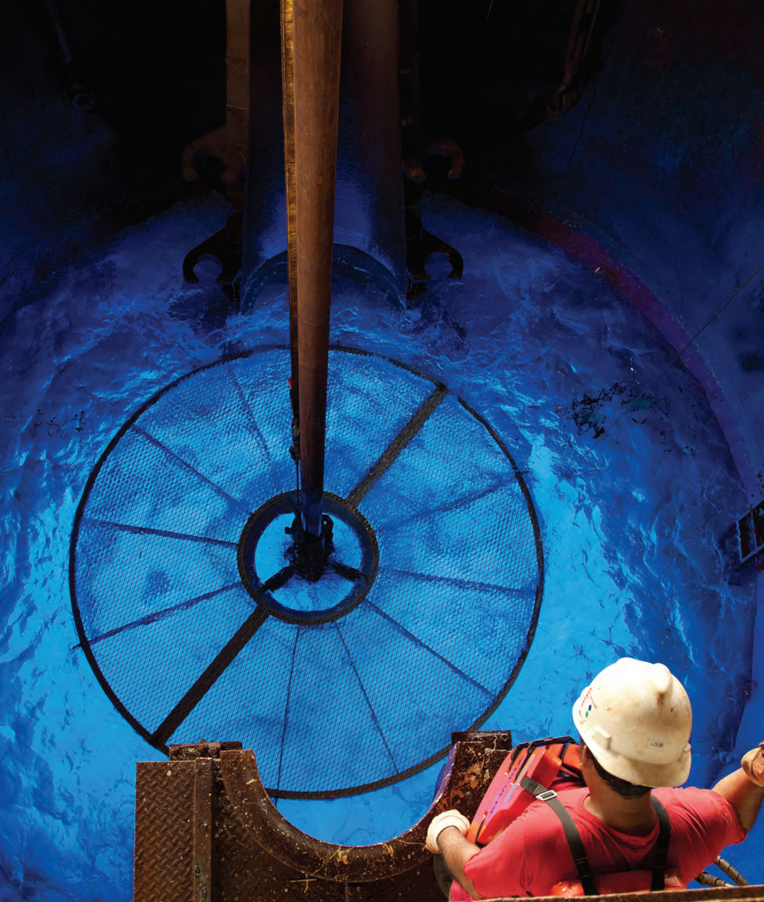
Lowering an ROV platform through the moonpool
