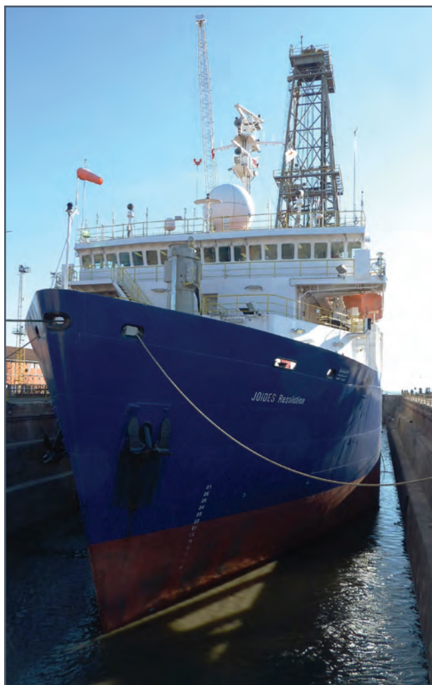
Floating the JOIDES Resolution off the drydock blocks
