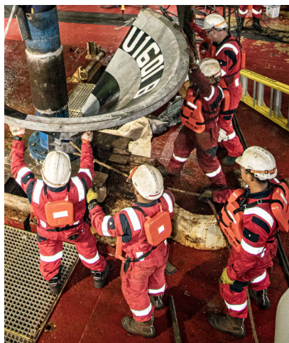
From left: Determining core splitting angle based on structures. Building a reentry cone around a short casing string. Shrunken Styrofoam cups after a trip to the seafloor.
