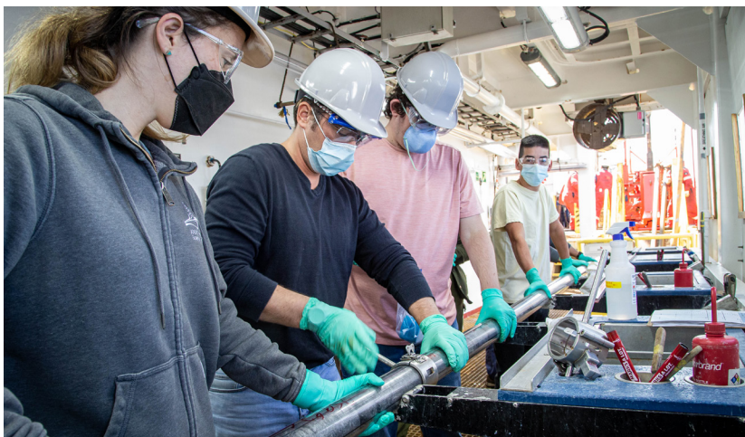
From left: Cutting a core into sections on the catwalk. A view of the JOIDES Resolution 's mast and derrick from the deck.
