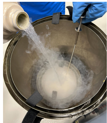
From left: A spectacular sunset framed by clouds. Pouring liquid nitrogen into the cryogenic container in the Paleomagnetism Laboratory.
