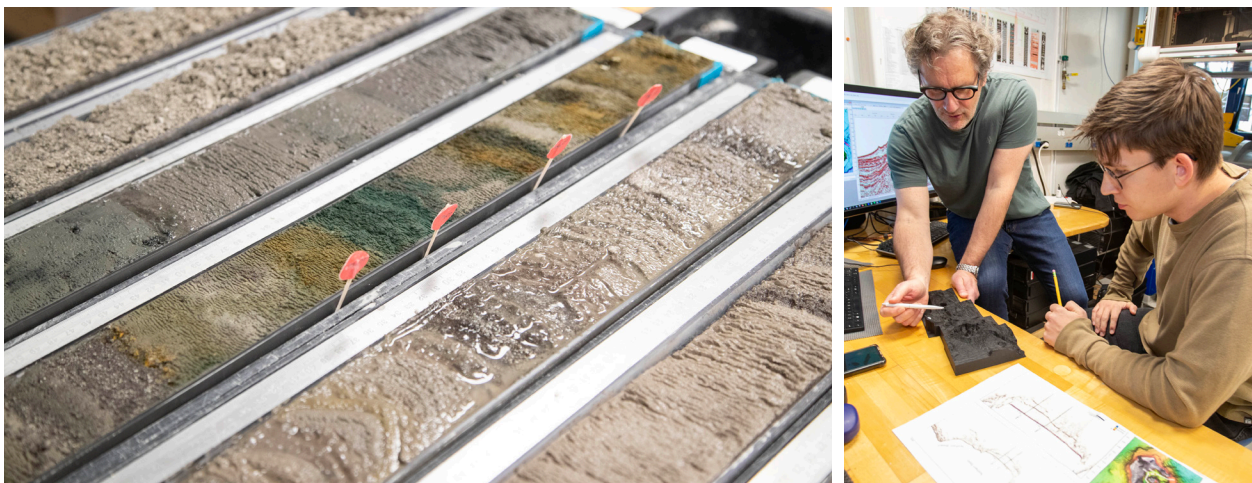
From left: Core sections on the sampling table. Comparing a 3-D model of the seafloor to seismic data collected precruise.
